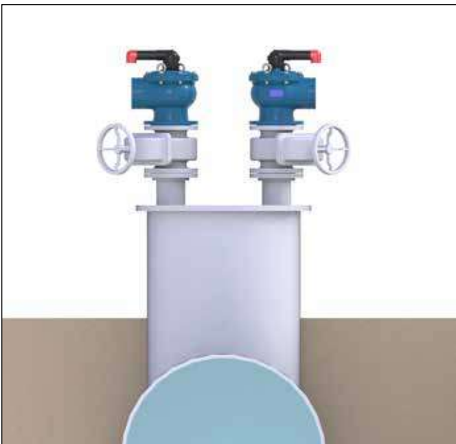
Two Air Valves on an Air Trap with separate Isolating Valves. Air Valve outlets face outward and the Isolating Valves at 45° to Air Valve outlets
