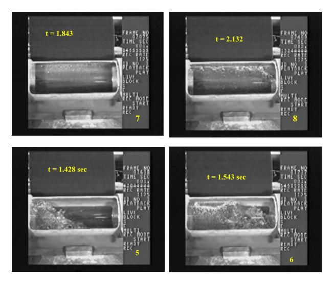
Figure 15: Views through a window, into the pipeline of the Fraunhofer UMSICHT surge test rig, showing water column separation and return and vapor cavity formation and collapse, down-stream from a fast closing shut-off valve. These views are frames from a video that was filmed at 1125 frames per second to capture the event and process.<sup>24</sup>
