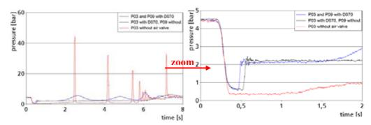
Figure 16: Graphs of pressure histories down-stream from the shut-off valve: red line, no air valve protection; black line, only the air valve at PO 3, down-stream from the shut-off valve, is active; blue line, both air valves, at PO 3 and at PO 9, at the top of the tower, are active. Dynamic D-070 air valves in both locations <sup>6</sup>
