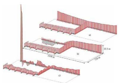
Figure 8: Snapshots from the simulation of power cut to pumps in the Production Block C2, a) steady state, b) minimum pressures with vaporous cavitation, and c) maximum pressures after cavity collapse
