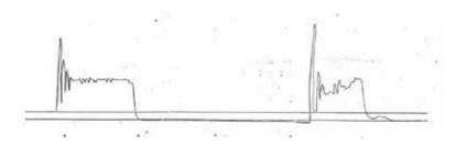
Figure 3: Joukowsky's pressure record exhibiting the initial upsurge at left, a down-surge, at water column separation, lasting about 1.15 seconds, and a second, higher upsurge <sup>3</sup>
