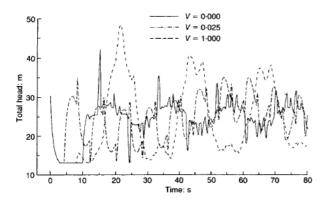
Figure 5: Variations of surge pressure at pump exit with and without an air pocket at
