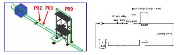
Figure 14: Faunhofer UMSICHT Division of Pipeline Technology surge test rig <sup>6/22</sup>
