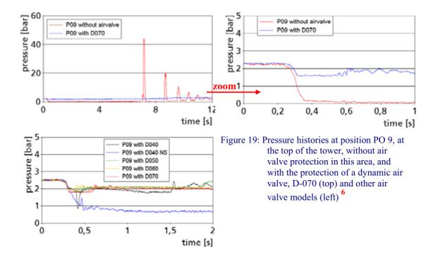
Application at this location was the least efficient. This shows that each location along the pipeline should be carefully assessed and the most efficient air valve should be chosen for that particular application. The D-040 without the non-slam accessory resulted in a down-surge of similar intensity, but, by far, a shorter duration. Though performing somewhat poorer than the other, larger orifice models at this location, the D-040, with its lower cost, may be more cost effective.
