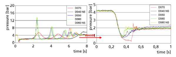
Figure 18: Comparison of pressure histories down-stream from the shut-off valve when different types of air valves are active at both PO 3 and PO 9 at the same time. The air valves at PO 3 and PO 4 are of the same type and size <sup>6</sup>
