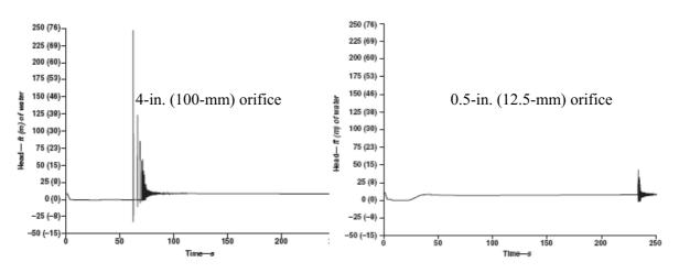
Figure 12: Surge analyses for secondary pressure surges due to final air release through 4 inch and 0.5 inch air discharge orifices <sup>9</sup>
